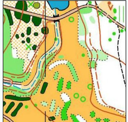
Sprint orienteering map with a scale of 1:4000, contour interval 2 m.
